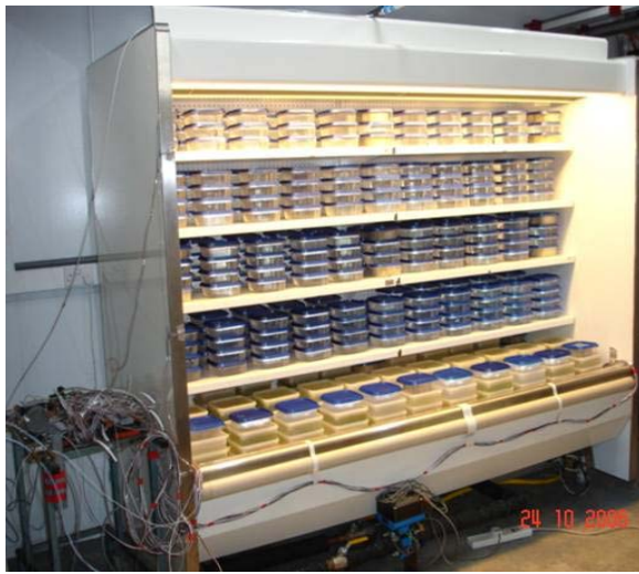
Figure 17: Secondary coil chilled food display cabinet.
